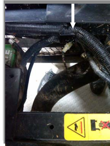
This wire harness is being cut by a chassis gusset
